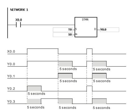
6. When the conditional contact X0.0 is followed by the b contact of Y0.3, the flashing currents pass through Y0.1 and Y0.2. When X10 is switched OFF, Y0.0, Y0.1, and Y0.3 are switched OFF, and T10 is reset to 0.
