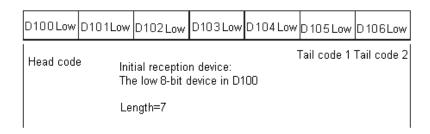
16-bit mode: The command which is edited is stored in the initial transmission device, and the command which will be sent include the head code and the tail code. When SM106/SM107 is OFF, the 16-bit data is divided into the high 8-bit data and the low 8-bit data.
