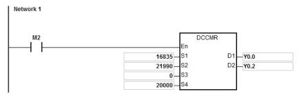
When PLC runs and M2 is ON, PLC will start to perform the relative-position circle drawing with the target reference frequency of 20kHz.
