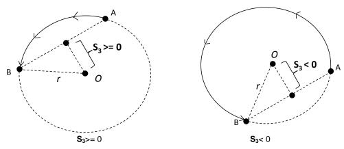
6. When X axis coordinate of target point B = 0 and Y axis coordinate >= 0, point B is defined as the point staying in QI of point A. Whereas, if Y axis coordinate < 0, point B is defined as the point staying in QIII of point A.
