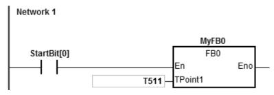
When VarBit1 in the FB0 is ON, the instruction TMR is executed, and TPoint1 (T511) starts counting. When the value of TPoint1 matches the setting value, VarOut is ON.
