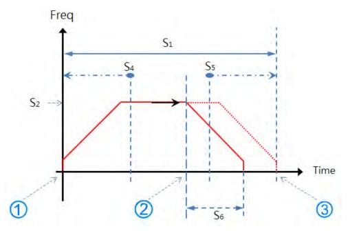
2. The mark alignment function is enabled in the ramp-up and target frequency and ramp-down sections.
