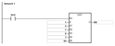
When the X0.0 is ON, the M0 will be ON too, meaning the daylight saving function is enabled.
