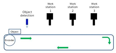
**Step 1:** using the input point X0.4 as the object detection interrupts, HC202 is the high-speed counter for the encoder and the output point Y0.0 as the initial output point for the work station to output.
