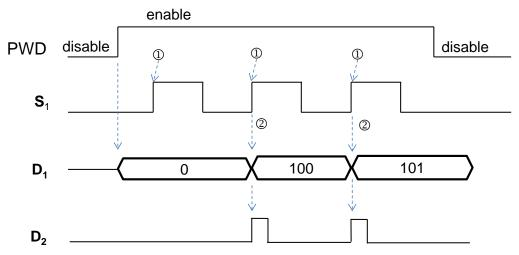
Figure 2 Detection mode when the value in S<sub>2</sub> is 4 or 5
