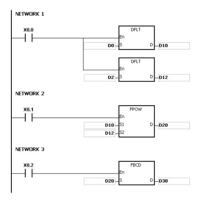
1. If the value in  $S_1$  is less than 0, the instruction is not executed, SM0 is ON, and the error code in SR0 is 16#2003.
