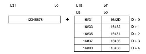
Suppose the value in L0 is 5126 and SM690 is OFF. When the PLC runs, the values are D0=16#3135, D1=16#3632, D2=16#0000.
