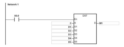
When the X0.0 is ON, the settings concerning the daylight saving will be stored in the assigned registers; see the examples below:
