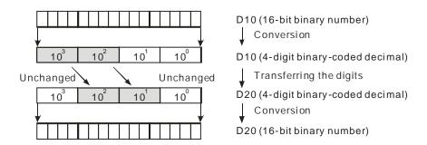
Suppose the number in **S** is K1234, and the number in **D** is K5678. After the instruction is executed, the number in **S** is 1234, and the number in **D** is 5128.
