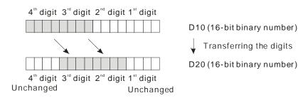
Suppose the number in D10 is 16#1234, and the number in D20 is 16#5678. After the instruction is executed, the number in D10 is unchanged, and the number in D20 is 16#5128.
