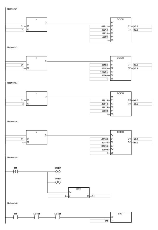
When PLC runs and M1 is ON, PLC will start the drawing of the first segment of the arc. D1 will increase by 1 whenever a segment of arc is completed and the second segment of the arc will start to
