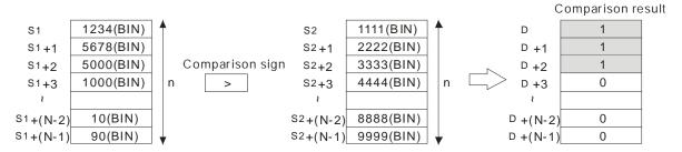
6. If the operand **S**<sub>1</sub> is a constant within the range between -32768 and 32767, the comparison will be as shown below.
