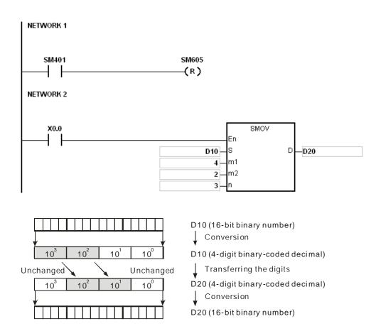
Suppose the number in D10 is 1234, and the number in D20 is 5678. After the instruction is executed, the number in D10 is unchanged, and the number in D20 is 5128.
