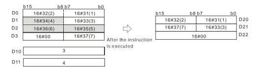
If the values in D10 and D11 are 5 and 4 respectively, the execution result is as follows. Owing to the fact that the number of characters which are deleted exceeds the range, the characters in D0~D3 starting from the fourth character to the last character are deleted.
