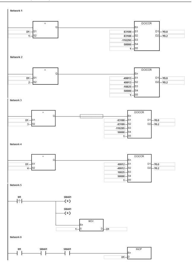
When PLC runs and M1 is ON, PLC will start the drawing of the first segment of clockwise arc with the frequency of 50kHz. D1 will increase by 1 whenever a segment of arc is completed and the second segment of arc will start to execute automatically. The operation pattern repeats until the fourth segment of arc is completed.
