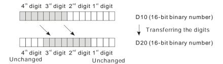
Suppose the number in **S** is 16#1234, and the number in **D** is 16#5678. After the instruction is executed, the number in **S** is 16#1234, and the number in **D** is 16#5128.
