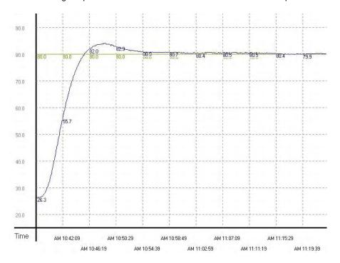
As the diagam above shows, after the parameters are tuned automatically, users can get a good temperature control result. It only takes about twenty minutes to control the temperature. When the target temperature changes from 80°C to 100°C, the result is as below.
