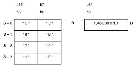
4. The string range in the device **S** for 16-bit instruction is 1~4 and for 32-bit instruction is 1~8.
