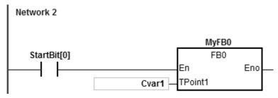
When VarBit1 in FB0 is ON, the instruction TMR is executed, and TPoint (CVar1) starts counting. When the value of TPoint1 matches the setting value, VarOut is ON.
