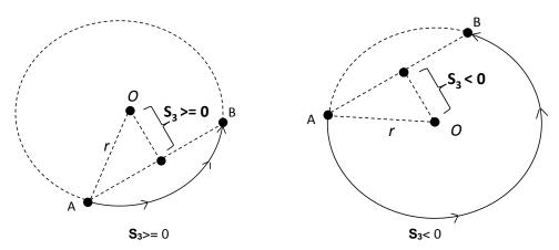
5. When the target point B is in QII and QIII of point A, the arc travel paths are shown as the solid lines in the figures below based the setting values in **S**<sub>3</sub>.
