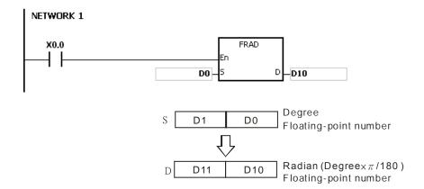
If the value in **S** exceeds the range of values which can be represented by the floating-point numbers, the instruction is not executed, SM0 is ON, and the error code in SR0 is 16#2013.
