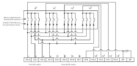
Note: The transistor output module AH16AP11T-5A is used in this example
