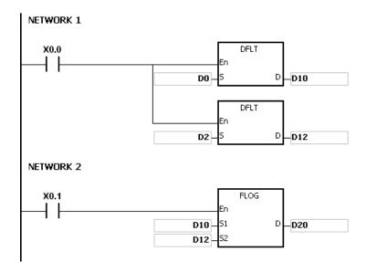
1. If the value in  $S_1$  is less than or equal to 1, or if the value in  $S_2$  is less or equal to 0, the instruction is not executed, SM0 is ON, and the error code in SR0 is 16#2003.
