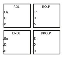
D : Device which is rotated
