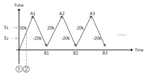
① DPPGB instruction is enabled. When  $S_1$  is 30,000 and  $S_2$  is -30,000, the motion will go toward the target position A1=30,000.
