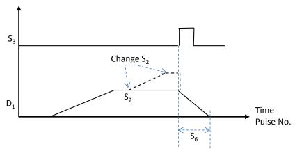
12. Refer to DDRVI instruction for the selection of pulse output devices for  $D_1$  and  $D_2$ . If the output points are not the recommended ones, the direction output  $D_2$  will be affected by the scan cycle.
