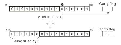
If  $\bf n$  is less than 0, or if  $\bf n$  is larger than 16, the instruction is not executed, SM0 is ON, and the error code in SR0 is 16#200B.
