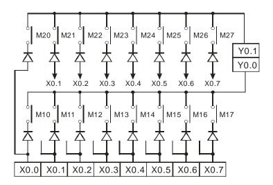
3. The eight input devices starting from X0.0 are connected to the two output devices starting from Y0.0 to form the two rows of switches. The states of the two rows of switches are read in the matrix scan, and stored in the devices starting from M10 specified by D2. That is, the states of the first row of switches are stored in M10~M17, and the states of the second row of switches are stored in M20~M27.
