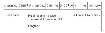
The data which the PLC receives from the external equipment includes the head and the tail code. Therefore, users have to be aware of the setting of a length.
