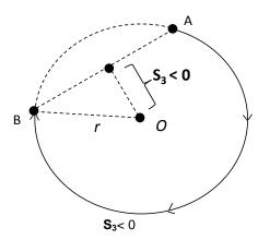
6. When of target point B, X axis coordinate = 0 and Y axis target coordinate >= 0, point B is defined as the point staying in QI of point A. Whereas, if Y axis target coordinate < 0, point B is defined as the point staying in QIII of point A.
