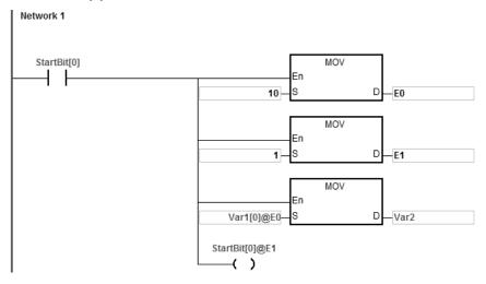
Additional remark: When users declare the variables in ISPSoft, and the variables are added to the contents of the registers to form the addresses to the actual data, users must note the addresses to prevent the program from being executed wrongly.
