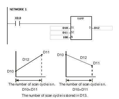
3. When SM686 is ON, and D12 is reaching the setting value in D11, the value in D12 will not be reset to 0, and SM687 is ON. Till the conditional contact is closed, the value in D12 will be reset to 0 and SM687 will be OFF. When SM686 is ON/OFF, the value in D12 changes as follows.
