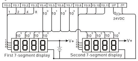
Note: The transistor output module AH16AN01T-5A is used in this example.
