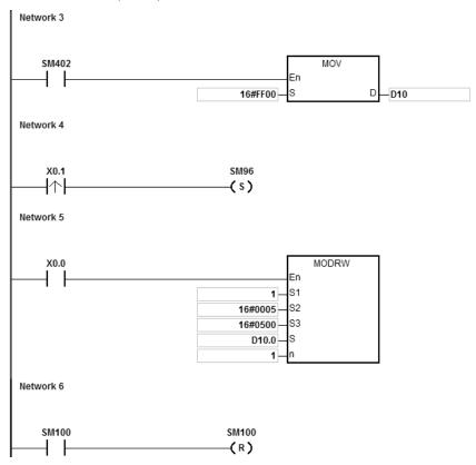
2. AS CPU module series is connected to the DVP-ES2 series PLC. D10.0 is ON and the Y0 of the DVP-ES2 series PLC is also ON. When SM96 and X0.0 are ON, the PLC can set the state of Y0.
