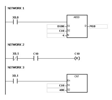
4. When the current value of C10 is within the range between the minimum value and the maximum value, M10~M13 are ON. Otherwise, M10~M13 are OFF.
