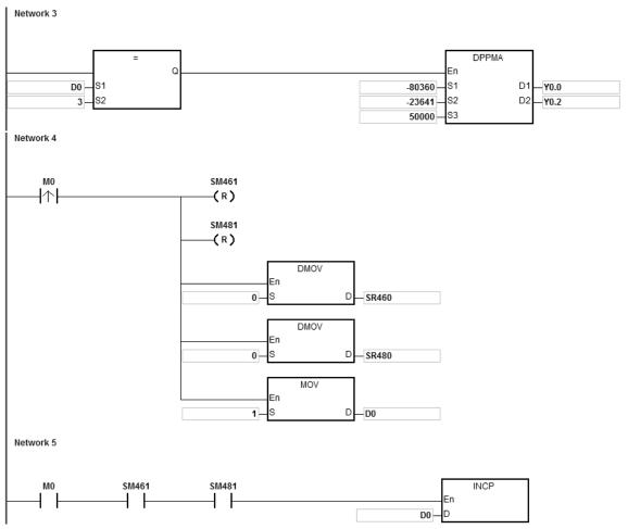
When PLC runs and M0 is ON, PLC will start to perform the first segment of 2-axis synchronized motion with the frequency of 50kHz. D1 will increase by 1 whenever a segment of 2-axis synchronized motion is completed and the second segment of 2-axis synchronized motion will start to execute automatically. The operation pattern repeats until the third segment of 2-axis synchronized motion is completed.
