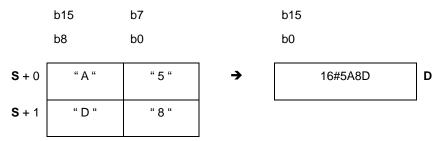
3. The operand **S** used in the 32-bit instruction occupies four word devices. If the value in **S** is a string and without the ending character 16#00, the conversion can be up to 8 digits (sign excluded). The hexadecimal ASCII code in **S** should be within the range between 00000000 and FFFFFFF. If **S** is a string, the string should be within the range between "0" and "FFFFFFFF."
