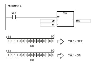
If  $\bf n$  exceeds the range, the instruction is not executed, SM0 is ON, and the error code in SR0 is 16#200B.
