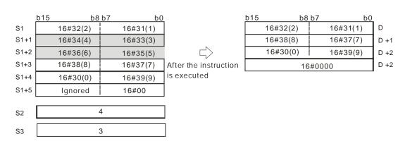
3. If the value in  $S_2$  is larger than the number of characters which can be deleted in the string in  $S_1$ , the characters in  $S_1$  starting from the character indicated by the value in  $S_3$  to the last character in  $S_1$  are deleted, and 16#00 is stored in D.
