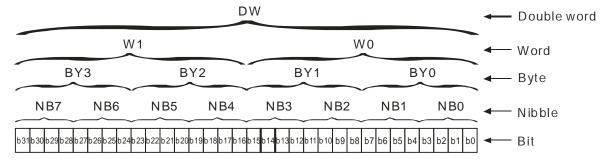
The PLC uses four types of values to execute the operation according to different control purposes. The functions of these values are illustrated as follows:
