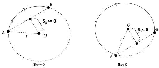
5. When the target point B is in QII and QIII of point A, the arc travel paths are shown as the solid lines in the figures below based the setting values in **S**<sub>3</sub>.
