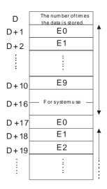
When X0.0 is ON, the value in D0 is set to 0, and the values in E0~E9 are transmitted to D1~D10. After the execution of FB0 is complete, the values in D1~D9 are read into E0~E9 via the instruction EPOP.
