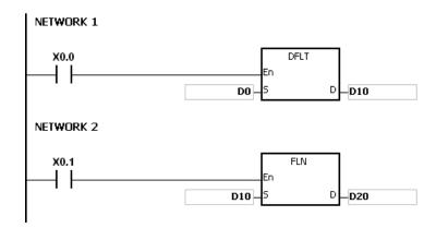
1. If the value in S is less than or equal to 0, the instruction is not executed, SM0 is ON, and the error code in SR0 is 16#2003.
