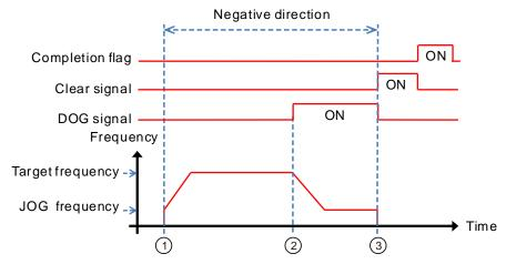
Function code 0+ the negative limit function enabling:
