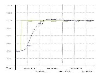
As the diagam above shows, when the target temperature changes from 80°C to 100°C, the parameters tuned previously still can be used to control the temperature. Besides, it does not take much time to control the temperature.
