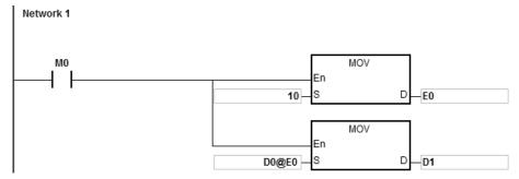
When M0 is ON, E0=10, E1=17, D1@E0=D (1+10)=D11, D11 is ON.
