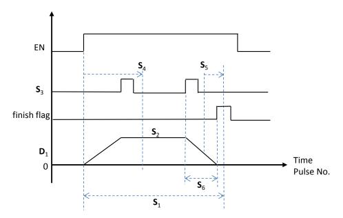
11. The target frequency S<sub>2</sub> of the instuction can be modified in the process of the pulse output. Since the number of output pulses in the ramp-down section has been set when the instruction is enabled, the timing diagram for changing the frequency is shown as the following dot line.
